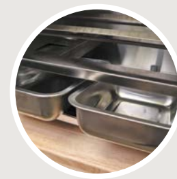
DUAL COLLECITON BASINS Individual basins to collect spent Bisquettes and renderings
